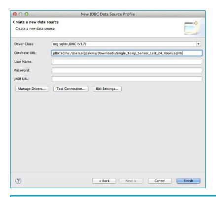
If the "org.sqlite.JDBC" Driver Class is not in the drop-down list, then it must be installed manually. The SQLiteJDBC driver is provided by RF Code on the Asset Manager Installation CD and in the downloadable image in the "Tools" directory. The SQLiteJDBC driver can also be downloaded from the following web page: https://bitbucket.org/xerial/sqlite-jdbc/downloads
