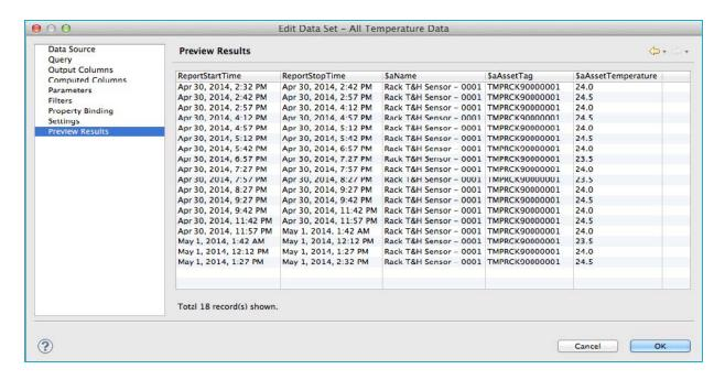
Notice in the image above that the \$aAssetTemperature (last column on right) is displayed in Celsius. The BIRT Report Designer can easily convert the Celsius reading to Fahrenheit. This is accomplished using the Computed Columns subtask.
