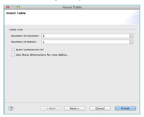
b. Enter 3 for the number of columns and 1 for the number of detail, then click **Finish**. The table is now created with a "header" row, a "details" row, and a "footer" row. The next step is to configure which information goes into which column of the details row.
