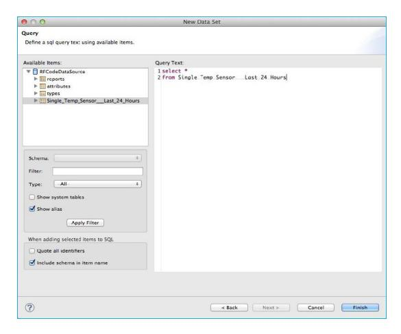
The Data Source in this example is simply a list of temperature values from one temperature sensors, so the query will be a straight-forward "select all" from the table.
